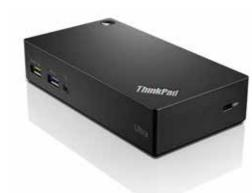
The ThinkPad USB 3.0 Ultra Dock has DisplayPort™ and HDMI™ digital video outputs that provide up to 4K2K video output (via DisplayPort™), and a new horizontal form factor that enhances the stability.
